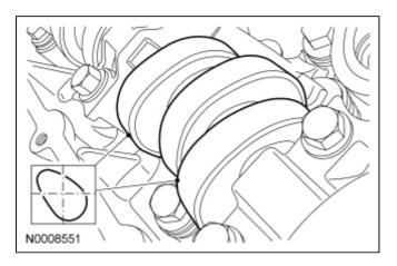
5. **NOTE:** Do not allow the valve keepers to fall off of the valve or the valve may drop into the cylinder. If a valve drops into the cylinder, the cylinder head must be removed. For additional information, refer to <a href="Cylinder Head">Cylinder Head</a> in this section.
